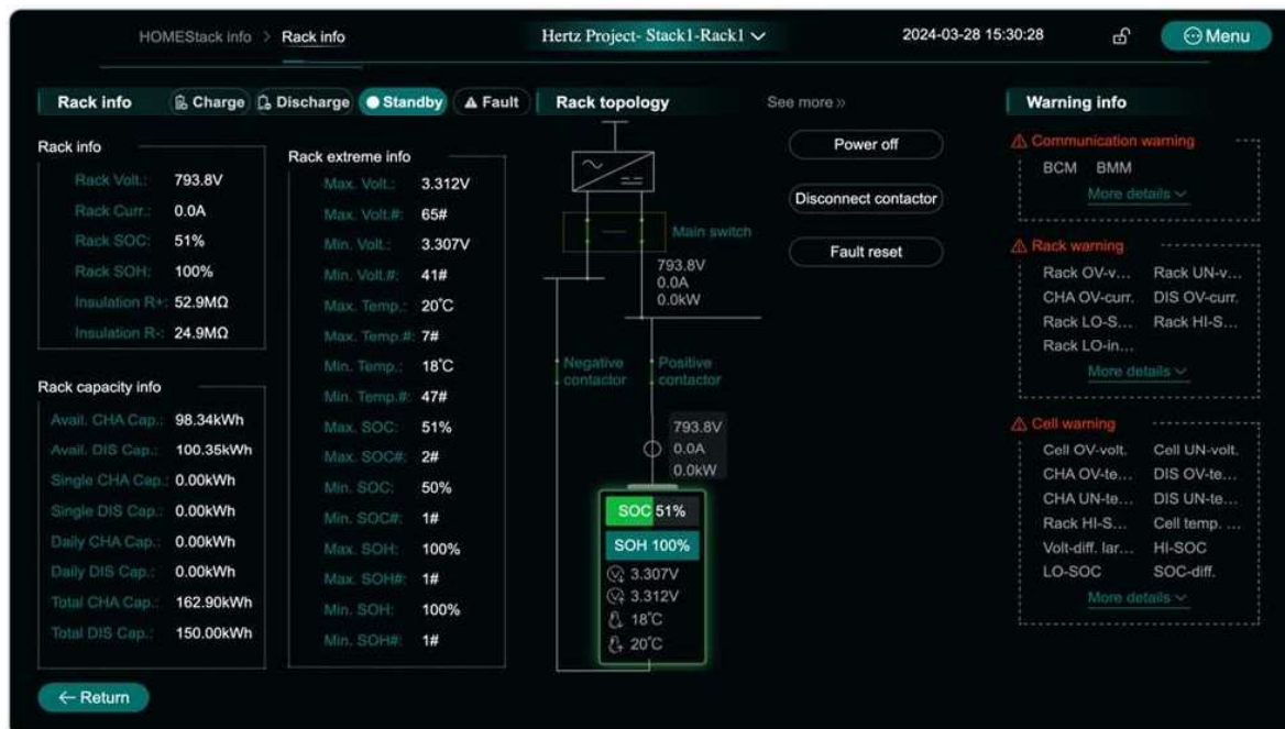
5.1-16 Battery stack subsystem interface
